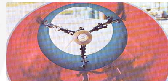
• Orbiter: coating equipment inside pipe
