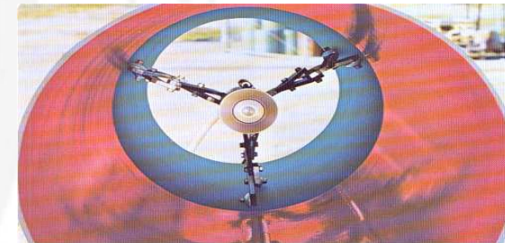
• Orbiter: coating equipment inside pipe
