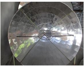
**Figure 40:** SK-14 Solar Cooker using cheaper Chinese-made reflectors
