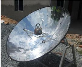
**Figure 41:** SK-14 Solar Cooker using expensive German-made reflectors Source: ASEIC (2011)
