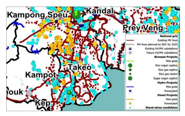
**Figure 35:** Grid Extension by Mini-grid and Standalone Systems (grid extension by 2020 in red, standalone villages by 2020 in blue, power plants in yellow)
