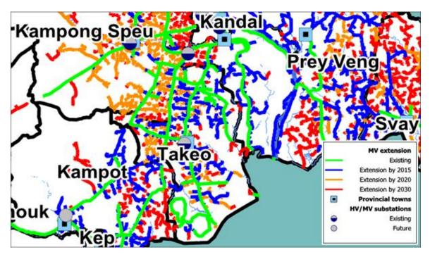
**Figure 34:** Grid Extension Plans to 2030 (green is existing, blue by 2015, orange by 2020, red by 2030) Source: IED, 2011
