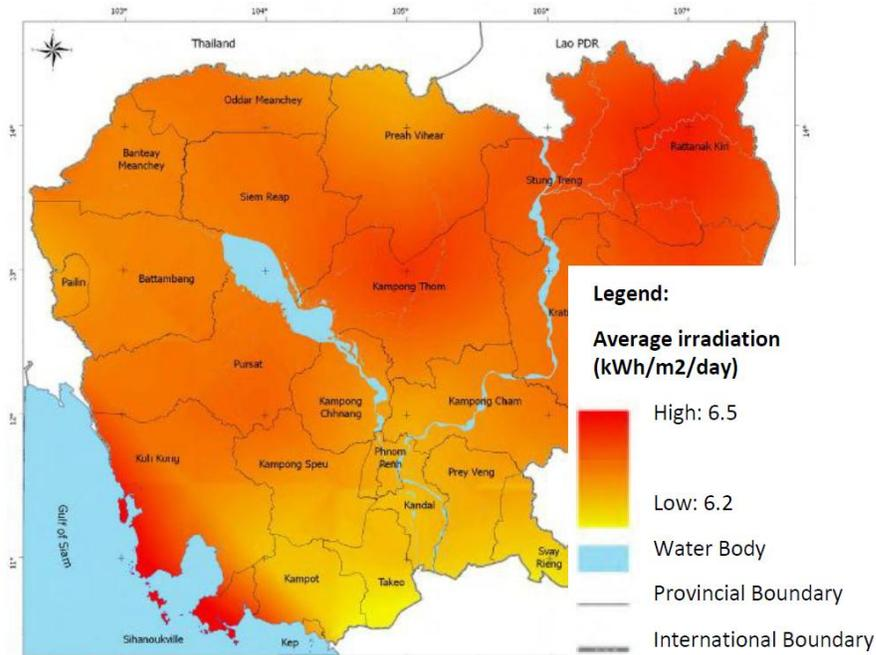
**Figure 5: Solar Irradiation Map of Cambodia**
