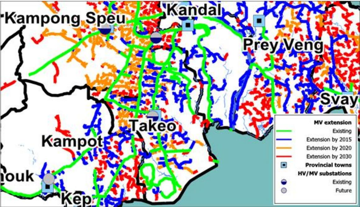
Figure 34: Grid Extension Plans to 2030 (green is existing, blue by 2015, orange by 2020, red by 2030)
