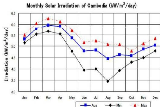
**Figure 4: Cambodia Monthly Solar Irradiation**
