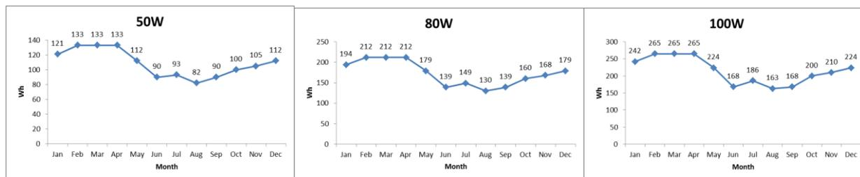
**Figure 19:** Quantity of Electricity Generated by a 50W/80W/100W Module (Wh/month)
